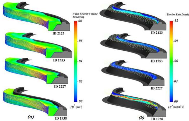
**Figure 7: Interesting Pareto Solutions (a) Volume-Rendered Velocity Magnitude (b) Erosion Map**
