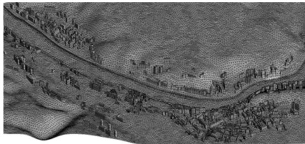
**Figure 2: Computational Domain and Surface Mesh**
