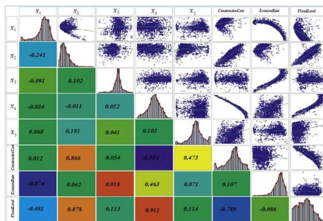
Figure 6: Scatter Matrix for Objective Functions and Design Parameters
