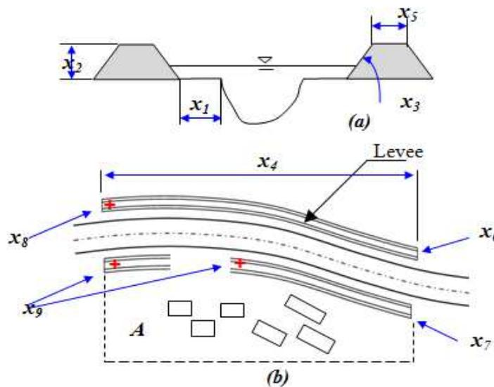
**Figure 3: Geometry Sketch and Design Parameters Employed for the Optimization.**
