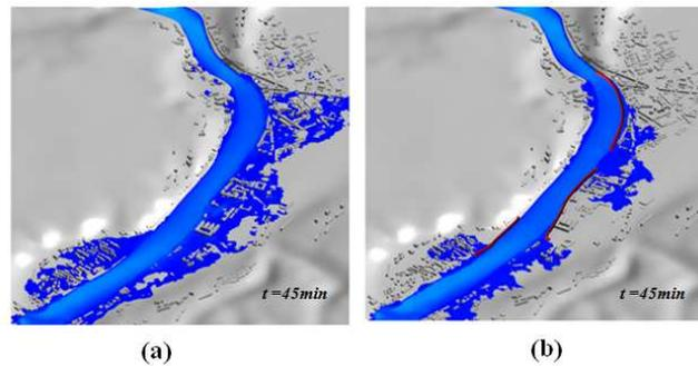
**Figure 8: Flood Propagation versus Time (a) not Protected, (b) Partially Protected by Optimal Levees**
