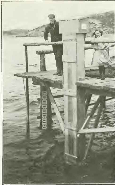
TEMPORARY TIDAL STATION showing a scale and tide column with shelter box on top which contains the Recording Instrument, at Bonne Esperance near Belle Isle Strait.
